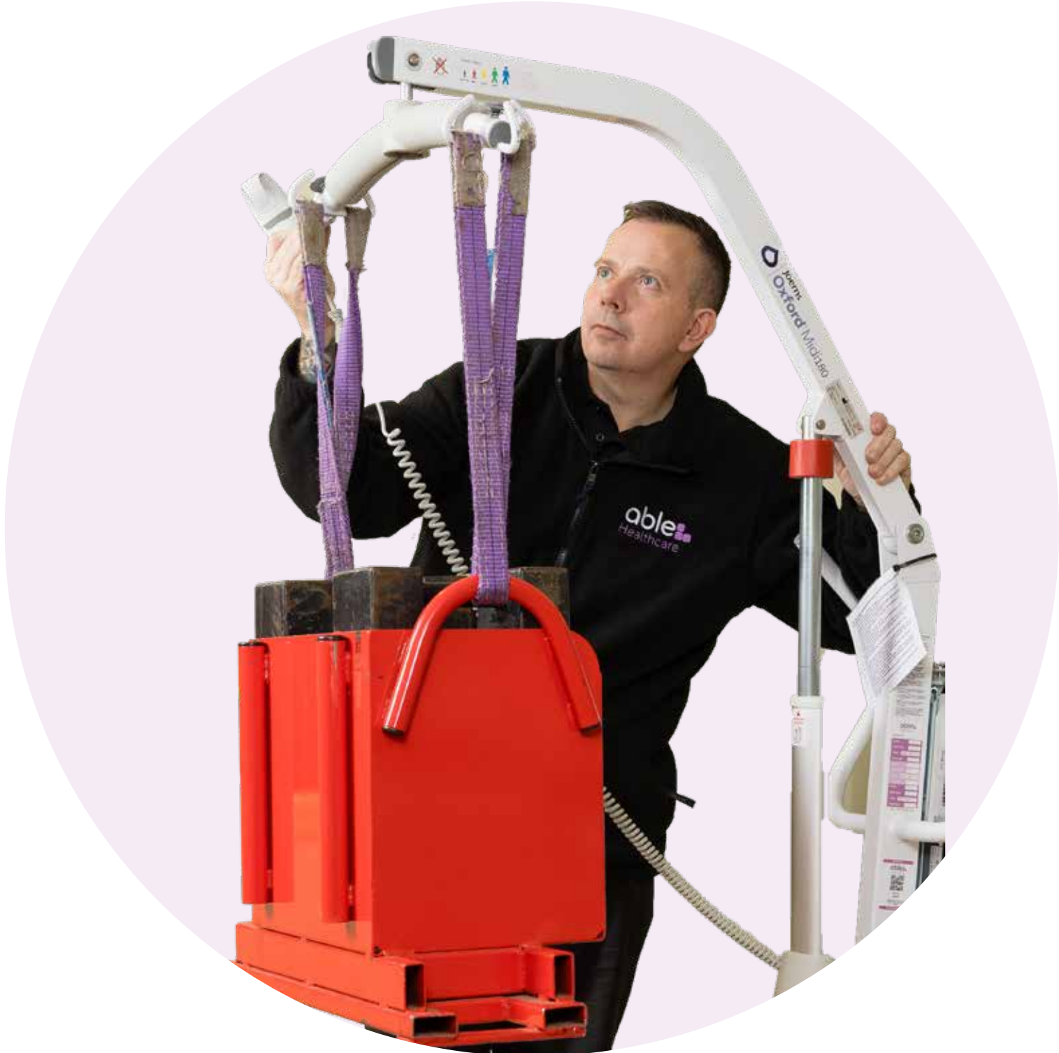
James, an Able Engineer, completing a full weight test (180kg) against a hoist.
